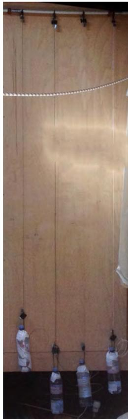
FIGURE 12 – Photo du test de fluage, filaments suspendus
