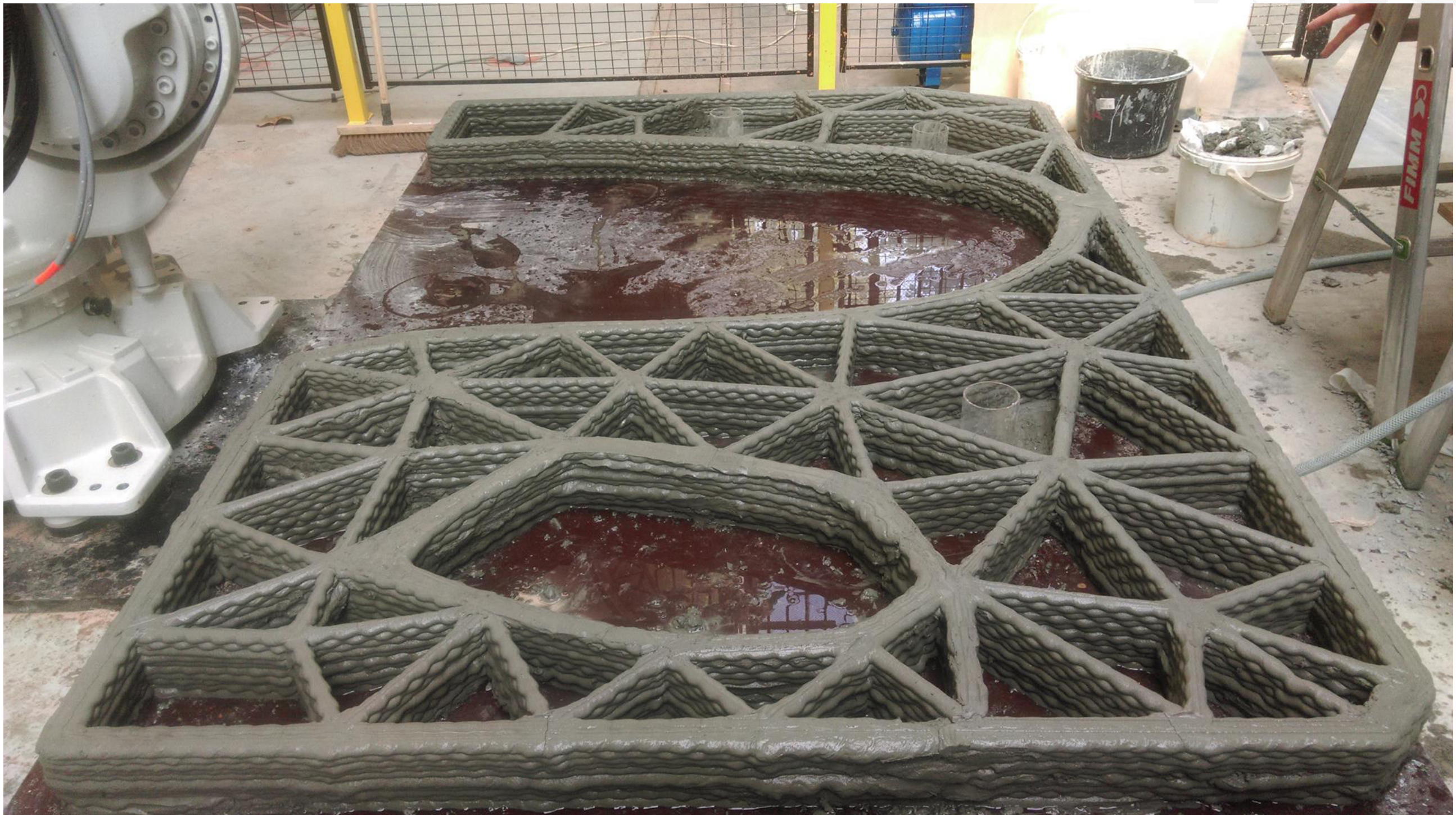
Large scale 3D printed prototype (DEMOCRITE 2015)
